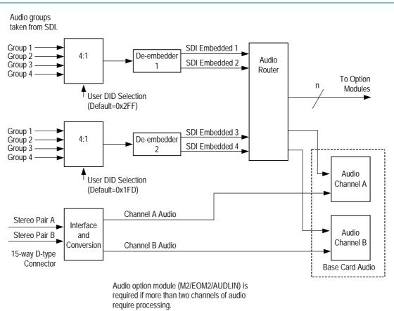
Figure G.3: Embedded Audio and Stereo Pairs
